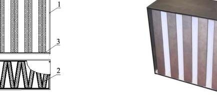
Fig. 1 Scheme of filter HFMF-F
